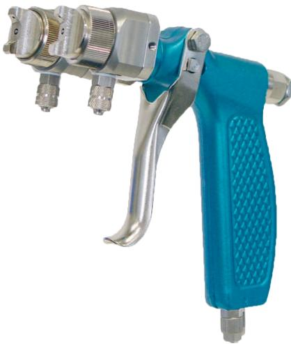
The mixing of both components happens within spray jet. In this way no early reaction between the components is possible. Mixing ratio of both components can be regulated individually by:
